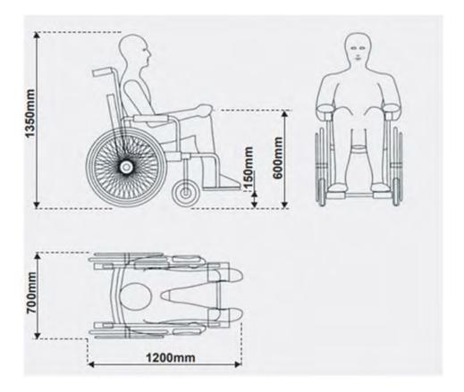
848. The reference wheelchair has: a total length of 1200mm including extra-long footplates total width of 700mm sitting height (from ground to top of head) of 1350mm. The reference wheelchair is bigger than most wheelchairs to ensure that enough room is provided for most wheelchair users.
